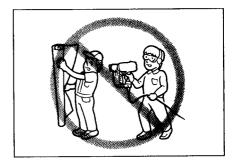
When the air hose is connected, do not carry the tool with your finger on the trigger or hand it to someone in this condition.
